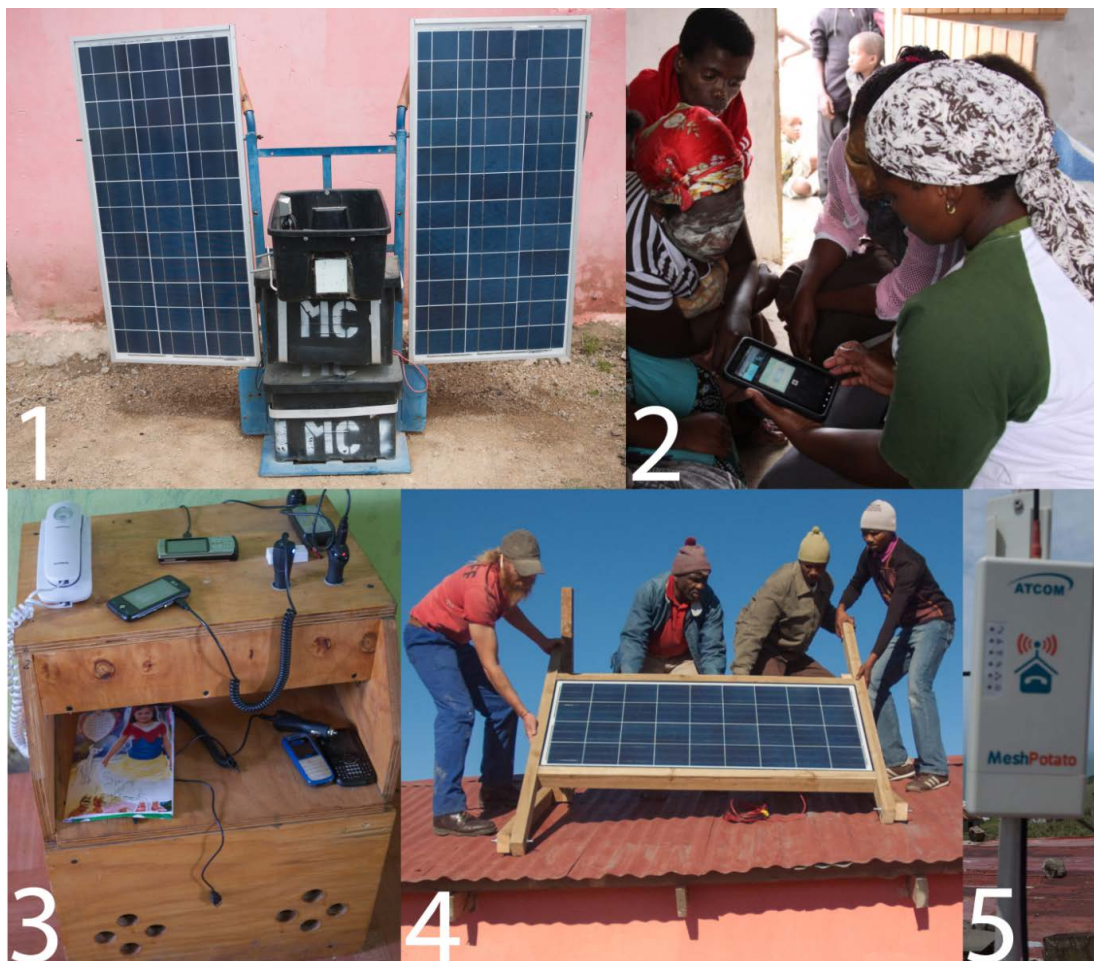
Figure 2. We trained participants to use solar cellphone Charging Stations (1) and Audio Repository (2) in workshops (upper) and to build and install wooden fixtures for the phone and charging apparatus (3) and for roof-top solar panels (4). The panels charge car batteries (in 3) to power the mesh nodes (5)
